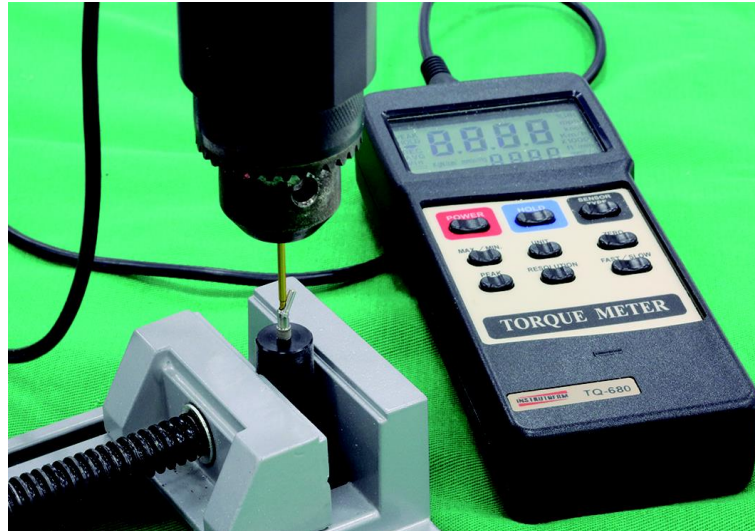
Figure 1 - Digital prosthetic ratchet (TQ-680, Instrutherm) used to tighten the prosthetic abutments to the implants.
