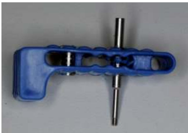
Figure 1 Guide pin inserted in the hollow tube positioned at the bite plate of the holder.
