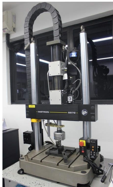
Figure 2. INSTRON 8872 Fatigue Testing System (Instron®, Norwood, Massachusetts, USA)
