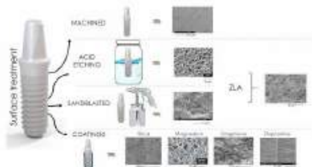
Fig. 1. Schematic and SEM images on different zirconia surface modifications: machined (1), acid-etched (2), air plasma (3), HA (4), and zirconia-coated (5).
